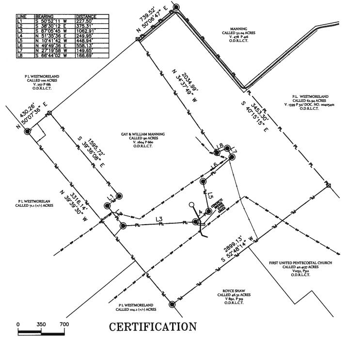
Basis of Bearings for this Survey is Grid North from GPS Observation TEXAS CENTRAL 4203 NAD83
