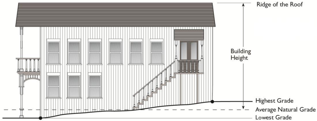
FIGURE 11.03.050(A): MEASURING BUILDING HEIGHT
