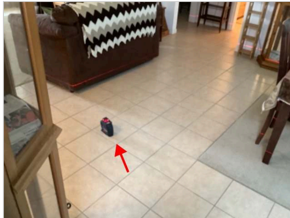
Floor levels taken
