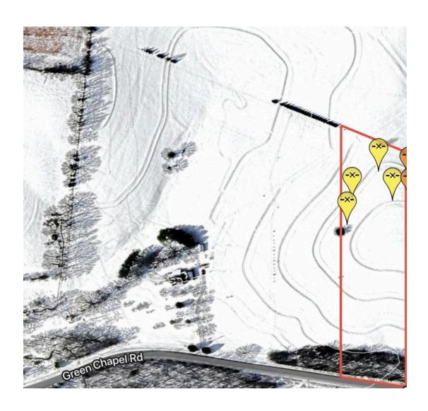
**SURVEYOR NOTE**: Grid stakes should extend at least 50 feet beyond the area(s) marked in the image(s) above. If, at the time of grid staking, the area(s) needs to be mowed, bush hogged, forestry mulched, or otherwise maintained please inform the customer immediately.
