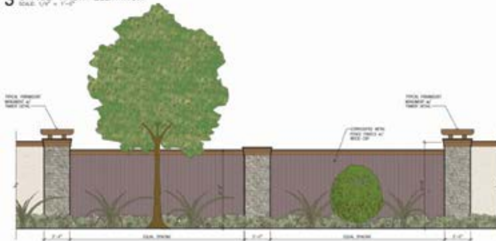
4 PERIMETER FENCE DETAIL #1 SCALE: 1/4" = 1'-0"
